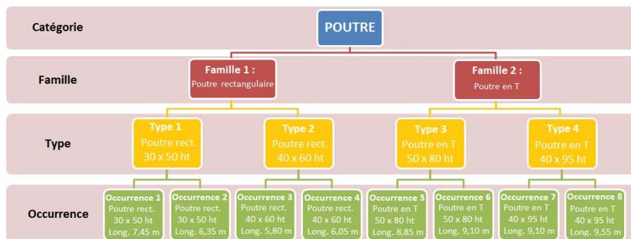
This hierarchy is fundamental to understand parametric drawing on REVIT. Each instance or element drawn on REVIT's interface includes in itself all inherited information. This information, in the form of parameters, allows us to automate the quantification, analysis and representation and also to instantly change the properties of each object.
